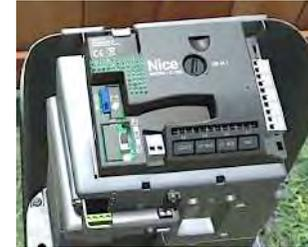
Selecting the gate's open direction with a switch.
